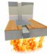
995 Fire Rated Pre-compressed Foam
